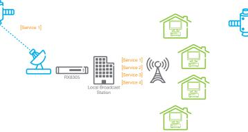
By additionally incorporating legacy DVB-S and MPEG-2 decoding this Multi-Format SD decoder provides flexible reception of a multiplex of satellite channels, descramble and decode a single service and interface into a local broadcast station through any of the unit's analog composite video, SDI digital video and ASI transport stream interfaces.
